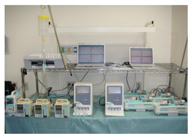
infusion pump with incorrect values, the test is repeated over 12 hours or more to confirm the flow rate (Fig. 4). Upon completion of the inspection, a flow rate inspection report is printed out and filed in the equipment control register. All inspected infusion and syringe pumps are marked with a sticker showing inspection completion in monthly different colors and are then available for rent.
