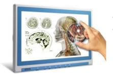
lying out on the glass sheet. Voltage is applied to this grid creating an <u>electrostatic</u> field. When the finger comes into contact with the screen it distorts the field at that point, measured as a change in <u>capacitance</u>. This change in charge can be measured extremely accurately and even a gloved finger can be sensed by PCT. The sandwiched sensor grid allows even two to ten finger touch points for pre-defined gestures like pinching,
