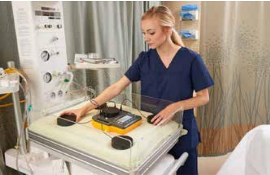
Pucks are used with the INCU II Incubator/Radiant Warmer to verify the performance of a radiant warmer
