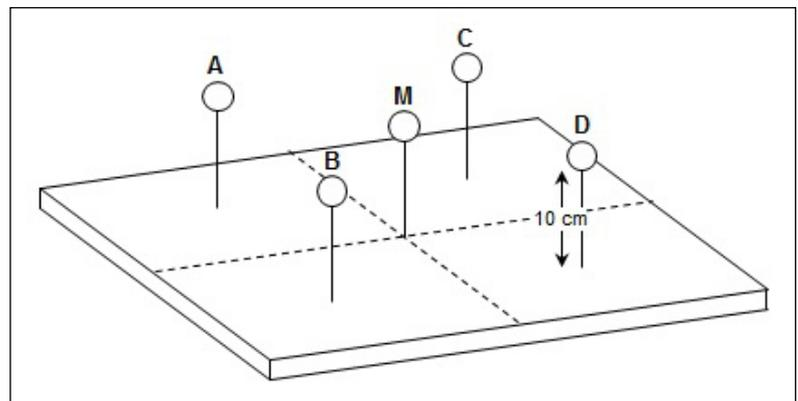
Figure 2. Air temperature probe height and placement on mattress
